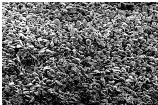
Scanning electron microscope pictures of the cross section of (A) a LiChrospher® HPTLC plate and (B) a HPTLC silica plate
